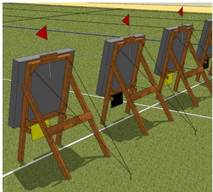
Figure 11. Target Buttress Rear View showing tie back
